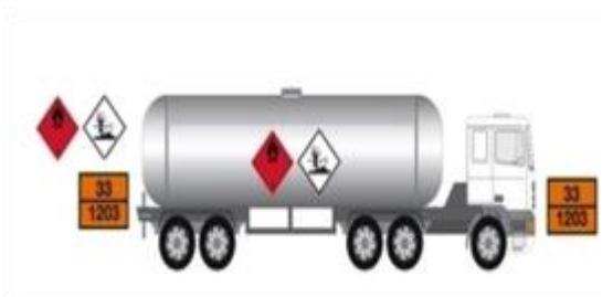
Tankers Carrying Dangerous Goods
